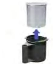
m) Remove the spray guard with the pacotizing blade and retrieve the pacotizing beaker from of the protective beaker.
