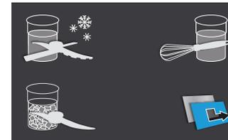
Utilizing the ON/OFF switch to power on the PACOJET 2, the display will show the PACOJET logo for several seconds. Immediately following, the home screen will load, which features 3 processing mode icons and an icon to access cleaning and machine settings functions. From this home screen, the PACOJET 2 can now be set/programmed for the processes required.
