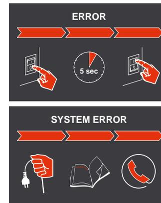
Power off the machine using the ON/OFF switch. After approx. 5 seconds, power on the machine. If the PACOJET logo is shown on the display, followed by the programmed processing mode, continue processing further beakers.
