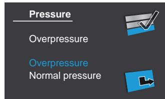
b) Presetting the overpressure function: Overpressure can also be deactivated by default using the arrows and the validation button.
