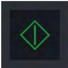
The START button is used to begin a processing cycle. Before a processing cycle can begin, a pacotizing beaker must be inserted within the protective outer beaker and mounted in place and the machine must be in ready mode.
