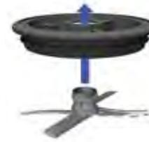
Grasp the pacotizing blade with two fingers on the corners between the blades. Place the pacotizing blade into the center hole of the spray guard, so that the hollow end fitting of the pacotizing blade snaps beyond the retaining tabs of the spray guard. Ensure that the flat side of the spray guard is facing downward against the blades.
