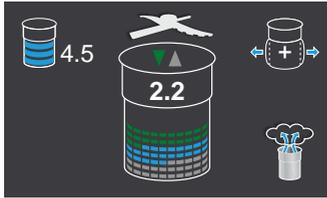
The display screen indicates the programmed portioning details prior to pacotizing and additionally, during pacotizing, the fill quantity of the beaker and the progress of the task. At the end of the task, the pacotized quantity and the non-pacotized quantity remaining in the beaker are also indicated. This display will clear when the protective outer beaker is dismantled from the machine.
