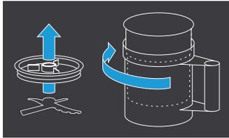
For further programming processing options within the mixing/whipping mode, either the pacotizing blade or the whipping disk (as supplied within the Pacojet Coupe Set package) must be positioned within the spray guard and correctly secured onto the magnetic, splined shaft of the PACOJET 2 machine. Then the pacotizing beaker and the protective outer beaker must be correctly mounted in the machine.
