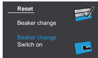
c) Resetting chosen processing options: There are two selection possibilities. PACOJET 2 can be set so that any chosen processing options will be reset to default settings either after each processing task (changing a beaker) or after powering off the machine using the ON/OFF switch.
