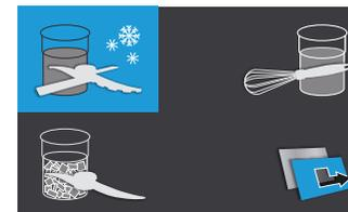
The 3 processing mode icons represent the 3 processing modes available : Pacotizing, Chopping/Cutting and Mixing/Whipping. When powering on the PACOJET 2 utilizing the ON/OFF switch, the home screen will appear after the PACOJET logo, on which the pacotizing mode is selected as the default.
