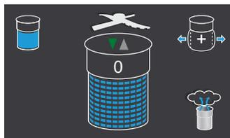
This display indicates the position and vertical movement direction of the pacotizing blade during a pacotizing cycle.
