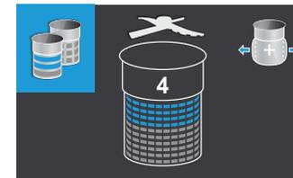
To pacotize food preparations into portions, a beaker’s contents filled to the maximum fill-line are divided into ten portions, each of which are further subdivided into ten decimal portions. In this respect, the total number of portions for a processing task may be programmed in full or decimal portions. This portioning feature has been calibrated according to the maximum fill-line volume of a beaker, not the actual content volume of a beaker.
