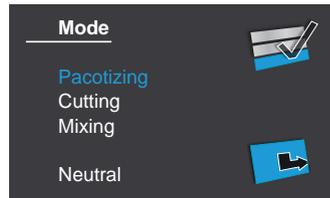
a) Presetting the processing mode: Using the arrow buttons to scroll through the menu and by pressing the validation button to confirm the selection, it is possible to program the presetting for each processing mode, as well as the presetting “Neutral”. Should the “Neutral” presetting be selected, the appropriate processing mode must be chosen prior to each processing task, as with this selection, no default processing mode is defined.
