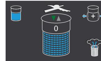
During a processing cycle with an activated “overpressure” setting, it is possible to depressurize the pacotizing beaker by pressing the appropriate selector button for “depressurize” on the control panel.
