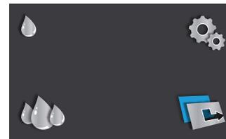
There are two cleaning cycle options on the left side of the display screen. Select the upper icon for a rinsing cycle or the lower icon for a full cleaning cycle. The settings functions can be accessed by pressing the selector button on the upper right of the control panel, adjacent to the “cog-wheels” icon shown on the display screen.
