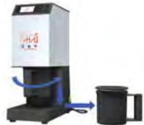
l) Demount the protective beaker by exerting counter clockwise pressure, i.e. from left-to-right-back, to withdraw it from the work position. The pacotizing blade and the spray guard will rest on the pacotizing beaker.
