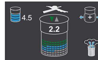
When the START button has been pressed, the PACOJET 2 will proceed through the chosen processing cycle fully automatically. Upon completion of the processing cycle, the shaft and pacotizing blade return to the start position, the beaker is depressurized automatically and the pacotizing cycle ends.
