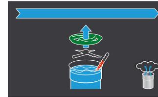
Rinsing the depressurization hose during a cleaning or rinsing cycle is possible by pressing the selector button for the depressurization function. Be sure to hold a cup under the hose outlet to collect any cleaning- or rinse-water that will be released.
