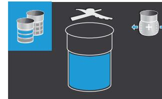
When the protective beaker is mounted correctly, the pacotizing settings are displayed immediately. The overpressure function is set by default for pacotizing prior to start and can be deactivated as required by using the selector or arrow buttons for "normal pressure" before start.
