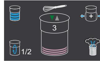
Should the same-cycle repetitions option be selected and programmed, the shaft and blade/disk will retreat to its starting position between beaker changes, or to the upper level of the selected approximate fill volume until the selected number of same-cycle repetitions is complete.
