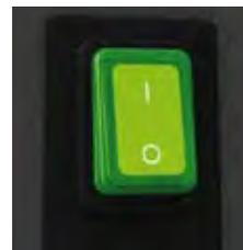
The ON/OFF switch is located toward the back of the lower, right side of the machine base. It is used to turn the machine on or off:
